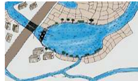
Bunds made of rocks constructed on one of the sides of the madaka to restrict the flow of water
